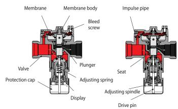
The HERZ-4006 SMART PIBCV has a pressure compensated upper part, so the maximum force required by the thermal drive is 100 Nm for all sizes of valve.
