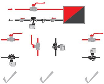
The valve is fitted in the return in any orientation. The arrow on the valve body should align with the direction of flow.
